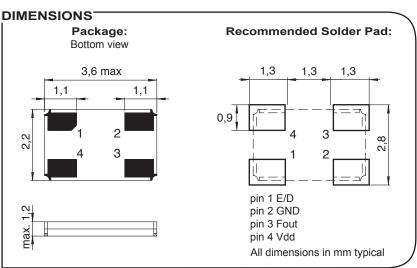
SMT Clock oscillator in ceramic package Fundamental quartz mode frequency High shock and vibration resistance
