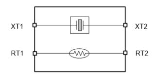
Note: RT2 shall be connected to GND is recommended
